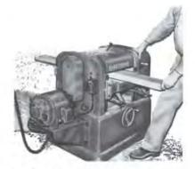
Feed Speed Adjustable from 15 to 37 feet per minute (76.20 mm to 187.96 mm) with variable speed pulley. Set quickly for every stock or finish requirement.
