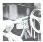
"Quik-Set" leature offers lever controlled table roll height adjustment from 0" to .040" (1.02 mm) at a touch. If you are tired of the 'push-pull" planing method. Quik-Set eliminates friction and constant under-the-table roll adjustments.
