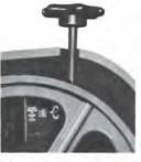
Eye level blade tension scale shows correct tension for different blade widths. Adjustable from front of machine.
