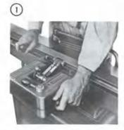
Extra Large Center-Mounted Fence plunger-locks at 90" with automatic stops at 45° right and left. Positive quick-lock in any other position. Glides easily and locks across full table width, or is removable for planing wide stock.
