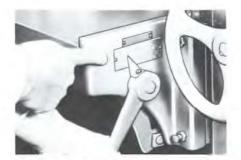
"Quik-Set" feature offers level controlled table roll height adjustment from 0" to .040" (1.02 mm) at a touch. Quik-Set eliminates friction and constant under-the-table roll adjustments.
