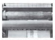
Sectional Infeed Roll corrugated 4" (101.60 mm) diameter, 2" 50.8 mm) cast iron sections mounted on milled alloy steel spline shaft. Reversible without damage. Each section has independent yield of 4" (6.35 mm), necessary in running strip stock of varying thickness without dangerous kickback.
