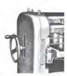
Convenient Bed-Adjustment Hand-Wheel — Acme-thread screws which operate in ball thrust bearings activates bed. Easyto-read thickness gauge. One-piece cast iron frame keeps perfect alignment.
