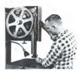
Counter-Balanced Guide Bar makes guide and blade adjustment safe and simple. Note telescoping guard completely enclosing blade above guide.
