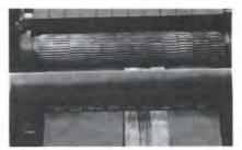
Sectional Inteed Rolls are corrugated, 4" (101.60 mm) diameter, 2" (50.8 mm) cast iron sections mounted on milled alloy steel spline shaft. Reversible without damage. Each section has independent yield of ¼" (6.35 mm), necessary in running strip stock of varying thickness without dangerous kickback.
