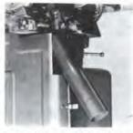
Exhaust Chute. This exhaust chute scavenges most of the dust and particles from inside the saw, reducing clean-out periods and improving saw performance.
