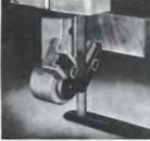
New upper and lower guide blocks with M-2 steel faced back-up bearings are standard with the Model 87. One set of %" (9.52mm) inserts only is supplied as original equipment.
