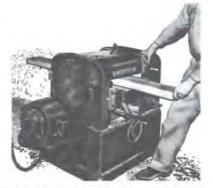
Feed Speed Adjustable from 15 to 37FPM (76.20mm/s to 187.96mm/s) with variable speed pulley. Sets quickly for every stock or finish requirement.
