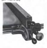
Fence Adjustment Fast and Sure from either side with Vernier control knob and top-reading front guide bar calibrations. Upper knob locks rear of fence. Fence is precision machined cast iron with tubular steel guide bars. Standard guide rails provide 25" (635.00 mm) cut to right of blade.
