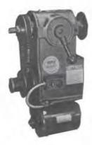
The Model 90 Lathe Drive System is a double reduction drive from the motor, through a jackshaft, to the headstock spindle. Isolation of the motor mount and the use of a jackshaft combine to minimize vibration.
