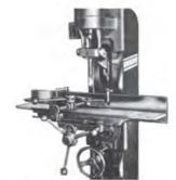
UNIVERSAL TABLE — assures complete flexibility for mortise cuts at any angle. Fast, simple 45° right or left tilting, 14" (355.60) vertical and 12" (304.80) longitudinal table adjustment.
