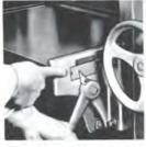
"Quik-Set" feature offers lever controlled table roll height adjustment from 0" to .040" (1.02 mm) at a touch. If you are tired of the "push-pull" planing method. Quik-Set eliminates friction and constant under-the-table roll adjustments.
