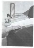
Optional miter attachment for straight and angular sanding.
