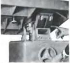
Heavy Duty 6" (152.40mm) Single-Action Trunnion for maximium rigidity. Adjust table 45° right, 15° left.
