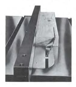
ADDED SAFETY: Blade tilts to left, away from Rip Fence, eliminates binding of material between blade and fence, thus helping to prevent "kickback" tendencies.
