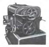
Belted Feed Drive Assembly is simple and trouble free. A combination of variable speed pulleys, V-belts, and heavy pitch gears provide smooth, dependable, feed rates without use of expensive and troublesome transmissions and pear-boxes.
