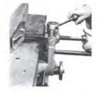
QUICK-ACTING ECCENTRIC CLAMP permits fast stock change with complete accuracy in high production operations.
