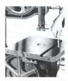
Side Takeout Slot for bandsaw blade elimi-nates necessity of split or narrow trunnions. Tapered pin keeps table surface flat,
