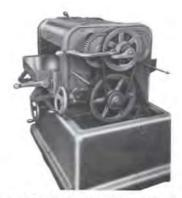
Beited Feed Drive Assembly is simple and trouble free. A combination of variable speed pulleys, V-beits, and heavy pitch gears provide smooth dependable feed rates without use of expensive and troublesome transmissions and gear-boxes.
