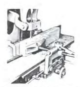
SLIDING TABLE RACK — with adjustable stops enables operator to make successive straight-line cuts with utmost precision on the #10 hollow chisel machine.
