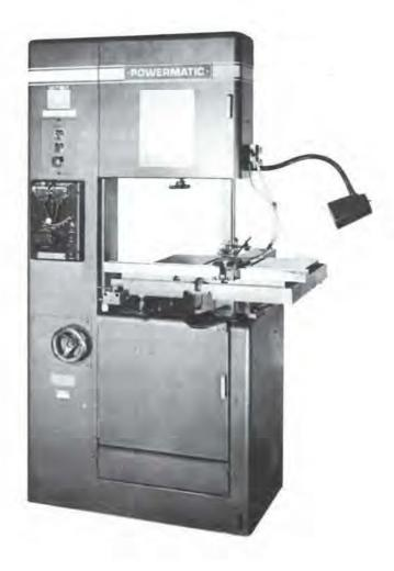
In addition to the rigidity and extra strength standard with Powermatic<sup>®</sup> bandsaws, the new "dynamatic" has improved on this feature with a new unitized steel frame. Deflection of the upper housing under full load is minimal.
