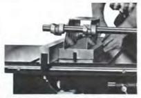
Hide away splitter swings out of the way behind saw when not required for dado operations.
