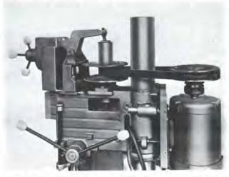
CHANGE SPEED INSTANTLY . . . CHECK SPEED INSTANTLY No belts to handle when you change spindle speed! Just a twist of the accurately-calibrated variable speed control lets you choose speeds instantly while machine is running. Extra wide speed range in one model. Increased accuracy and bit life in all drilling operations.
