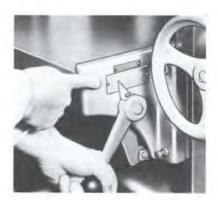
"Quik-Set" feature offers lever controlled table roll height adjustment from 0" to .040" (1.02mm) at a touch. Quik-Set eliminates friction and constant under-the-table roll adjustments.
