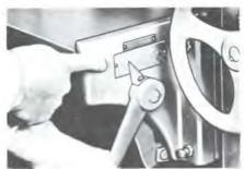
"Quik-Set" feature offers lever controlled table roll height adjustment from 0" to .040" (1.02 mm) at a touch. Quik-Set eliminates friction and constant under-the-table roll adjustments
