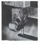
New upper and lower guide blocks with M-2 steel faced back-up bearings are standard with the Model 87. One set of %" (9.52mm) inserts only is supplied as original equipment.
