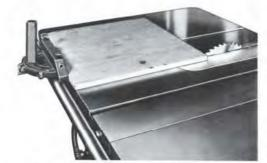
\*Extra Cut-Off Capacity table in front of blade is full 21" (533.40 mm) at 1" (25.40 mm) cut.
