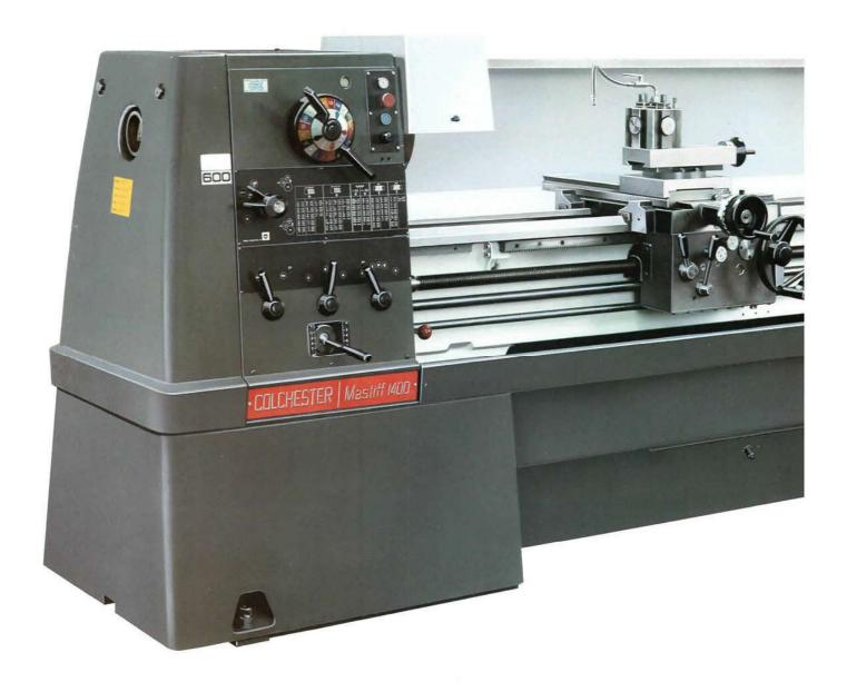
The Colchester Mastiff 1400 is a 535mm (21in) Swing Centre Lathe with a between centres capacity of up to 3 metres (120in). The heavy duty spindle arrangement makes the machine ideal for both production and repair work applications on heavier workpieces.
